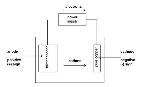
(a) Explain the chemical principles of an electrolytic cell.
